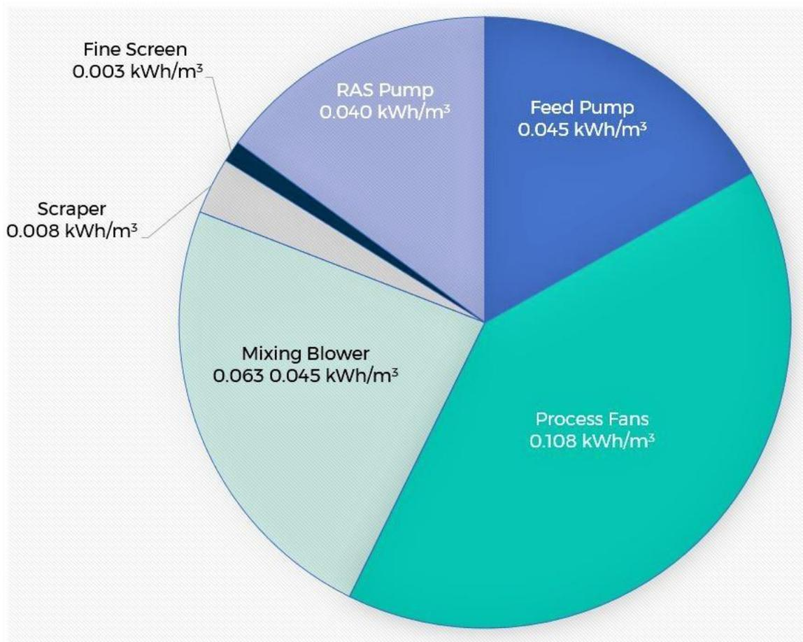
MABR plants use 0.267 kWh/m<sup>3</sup> of wastewater treated, a 61 percent reduction in energy use compared to a small nitrifying conventional activated sludge secondary treatment plant.
