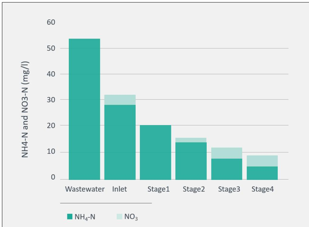
**MABR module in Stage 1 is operating at the highest nitrification rate but produces zero nitrate – it is all denitrified by the suspended biomass. Modules in Stages 2 and 3 continue the treatment. Effluent ammonia concentration out of polishing Stage 4 (containing no module) is less than 5 mg/L, and TN is less than 10 mg/L.**
