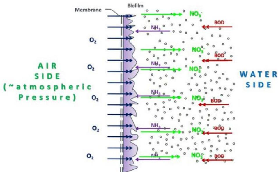
Oxygen diffuses through the membrane (known as passive aeration) to feed a nitrifying biofilm on the membrane's exterior surface, consuming oxygen and creating anoxic conditions beyond that are ideal for denitrification to occur.
