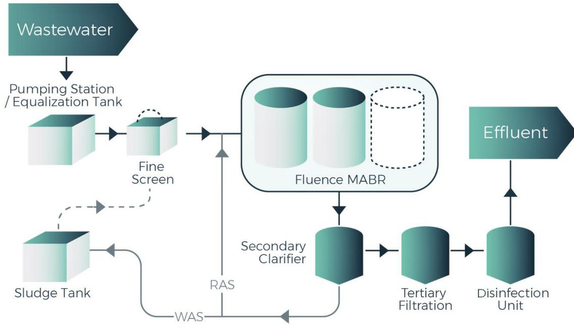
Aeration processes used to degrade organic matter represents anywhere from 25 to 60 percent of a traditional wastewater treatment plant's energy expenditure. Using passive aeration, MABRs demonstrate a dramatic 87 percent reduction in aeration energy consumption compared to conventional activated sludge (CAS) processes that employ diffusers and high-powered blowers (see table below).
